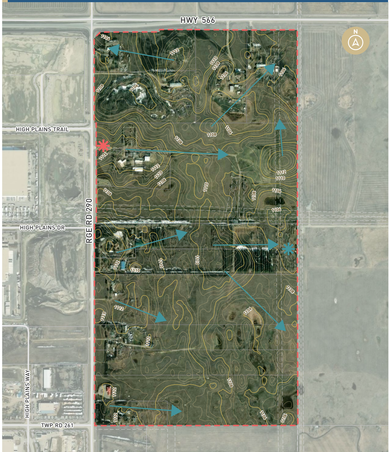
FIGURE 7 Topography and Existing Surface Drainage
