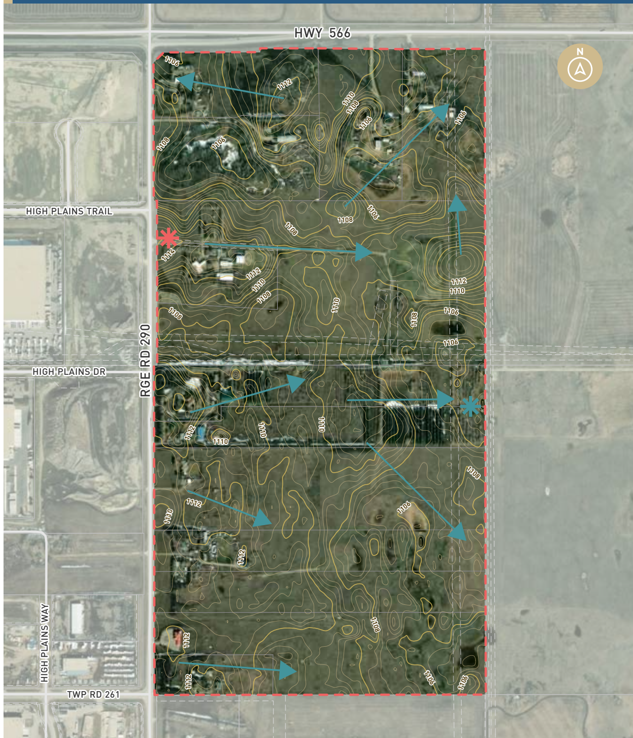
FIGURE 7 Topography and Existing Surface Drainage
